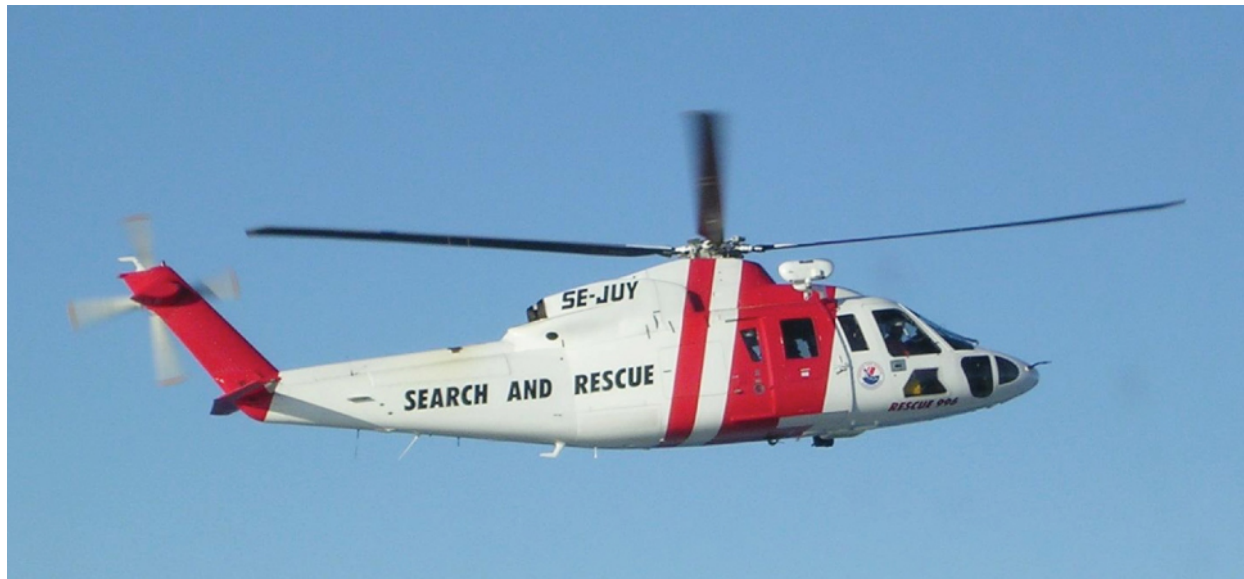
Figure 11.1 A helicopter has its main lift blades rotating to keep the aircraft airborne. Due to conservation of angular momentum, the body of the helicopter would want to rotate in the opposite sense to the blades, if it were not for the small rotor on the tail of the aircraft, which provides thrust to stabilize it.
