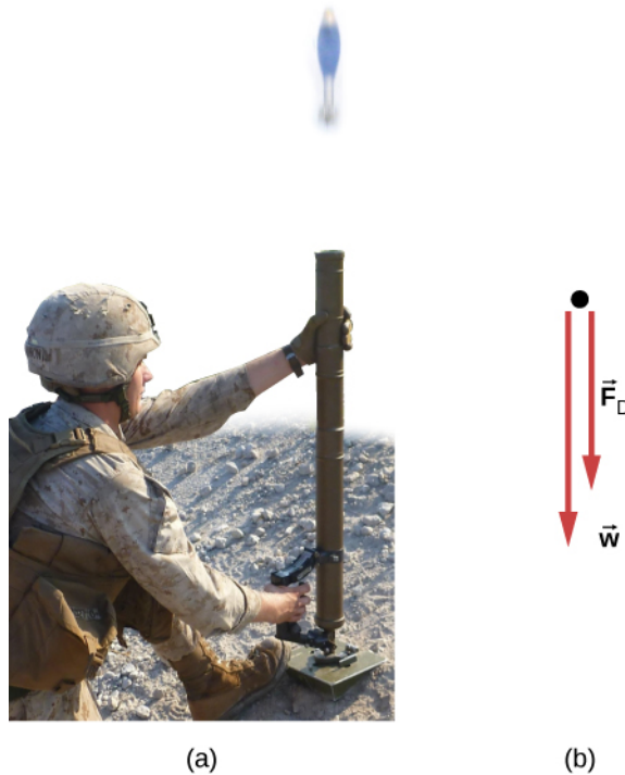
Figure 6.9 (a) The mortar fires a shell straight up; we consider the friction force provided by the air. (b) A free-body diagram is shown which indicates all the forces on the mortar shell.
