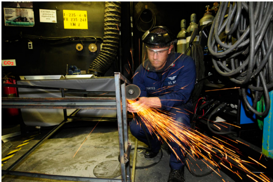
Figure 10.17 The rotational kinetic energy of the grindstone is converted to heat, light, sound, and vibration. (credit: Zachary David Bell, US Navy)
