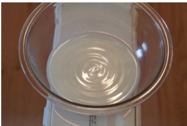
Figure 16.25 Standing waves are formed on the surface of a bowl of milk sitting on a box fan. The vibrations from the fan causes the surface of the milk of oscillate. The waves are visible due to the reflection of light from a lamp.
