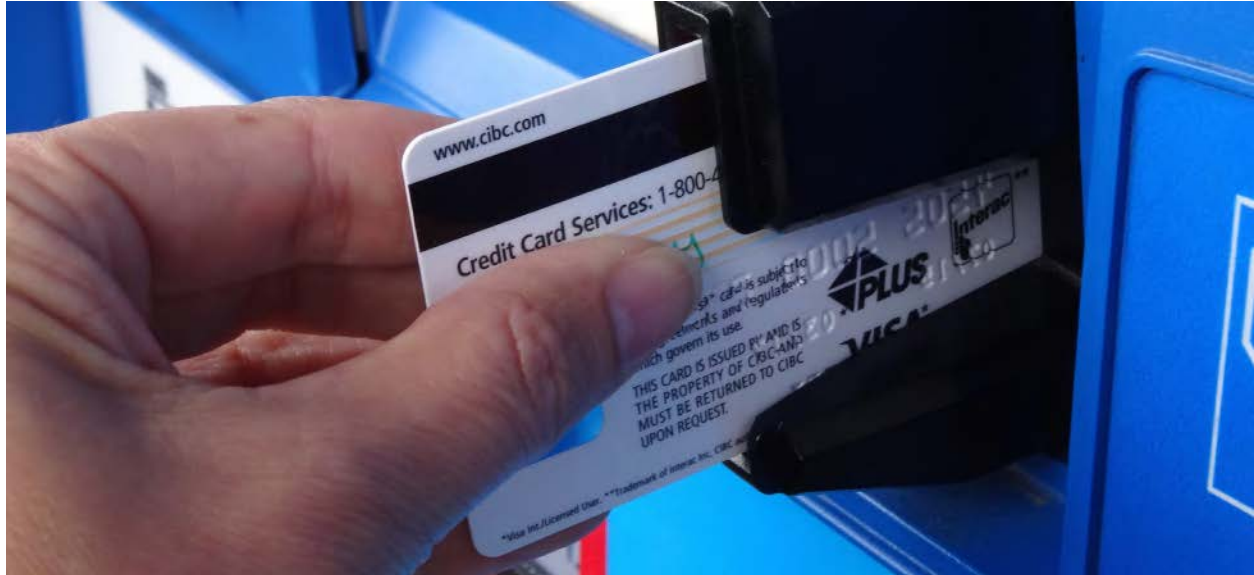
Figure 13.1 The black strip found on the back of credit cards and driver's licenses is a very thin layer of magnetic material with information stored on it. Reading and writing the information on the credit card is done with a swiping motion. The physical reason why this is necessary is called electromagnetic induction and is discussed in this chapter.
