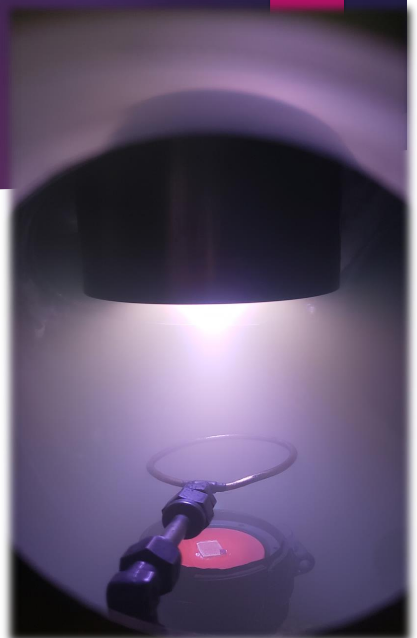
Fig 10. Sputtering Process. a) Substrate in the heater . b) Pre-sputtering time. c) Sputtering time
