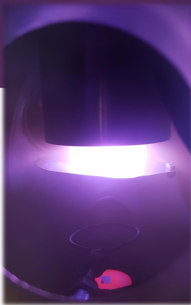
Fig 10. Sputtering Process. a) Substrate in the heater . b) Pre-sputtering time. c) Sputtering time
